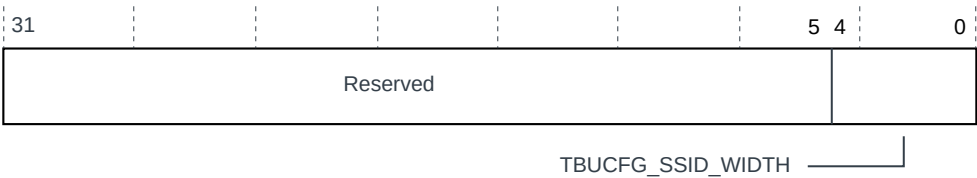
Figure 7-48: TBU_SYSDISC7 register bit assignments
