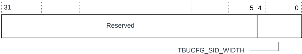
Figure 7-47: TBU_SYSDISC6 register bit assignments
