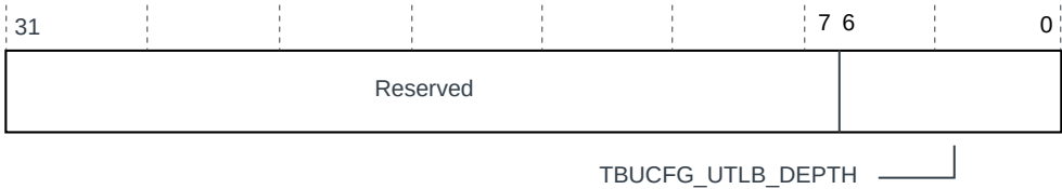
Figure 7-44: TBU_SYSDISC1 register bit assignments
