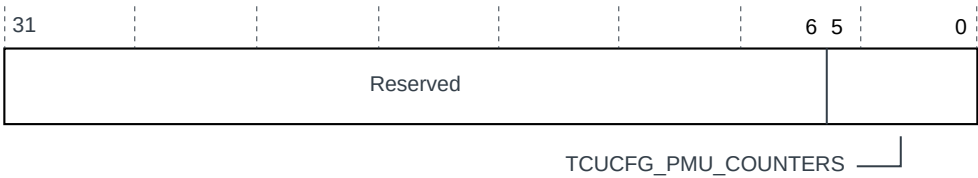
Figure 7-22: TCU_SYSDISC10 register bit assignments
