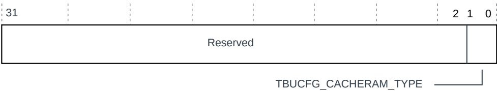
Figure 7-52: TBU_SYSDISC14 register bit assignments
