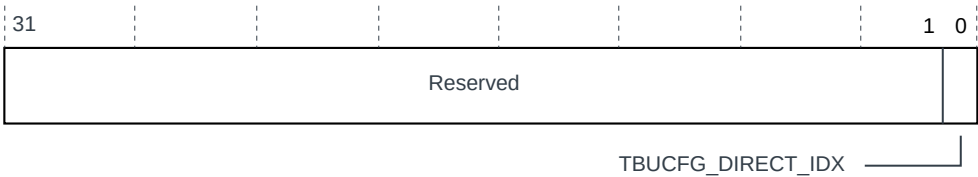
Figure 7-49: TBU_SYSDISC8 register bit assignments
