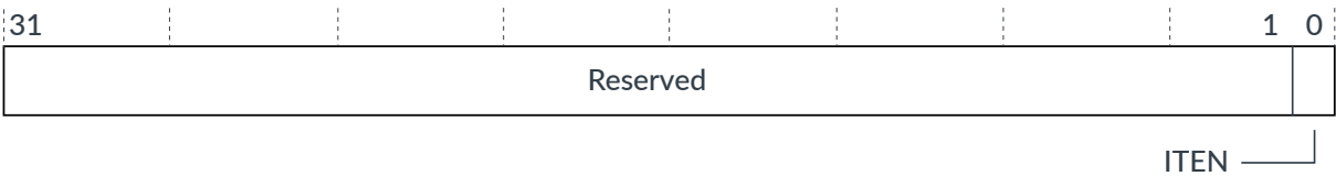
Figure 7-36: ITEN register bit assignments
