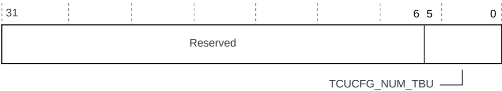
Figure 7-21: TCU_SYSDISC9 register bit assignments
